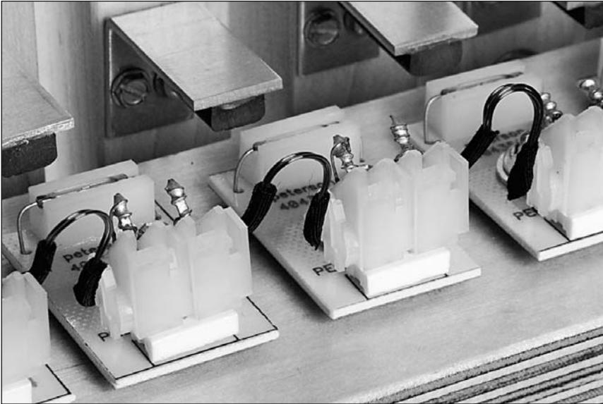
Peterson's improved Reed Switch Pedal Key Contact System now features a small, separate circuit board for each note. This allows the contact system to be installed either near the toe end of each pedal key, or on a cross member that may be fabricated under the center of the keys.
