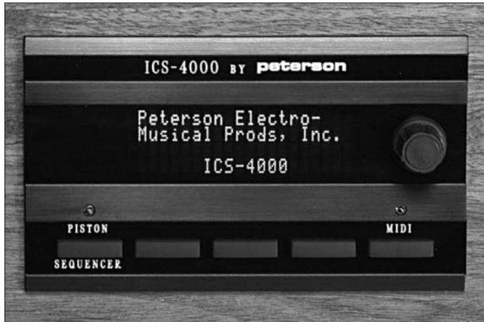
The Peterson ICS-4000™ combines an unprecedented number of available coupling, unification, combination action, and MIDI functions into a single software-driven system that may be customized for virtually any pipe organ application. Never before has such a powerful yet easy-to-use control system been available to pipe organ builders and rebuilders.
