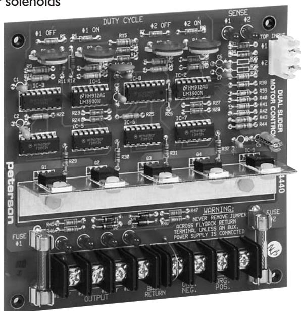
Separate power adjustment for on and off direction of each solenoid.
