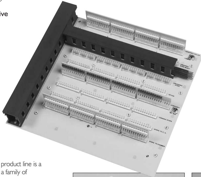
The foundation of Peterson's product line is a proprietary cabling method and a family of disconnectable junctions and connectors that literally revolutionized the manufacture of modern pipe organs. This concept greatly improves the practicality of completely assembling, wiring, testing and troubleshooting a pipe organ at an organ builder's facility before moving the organ to its installation site.
