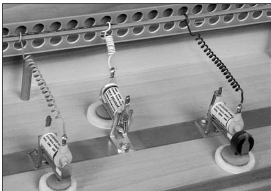
A toe board using the Buss Strip Mounting Kit and Keying Wire Spreader Kit.
