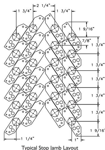
The Peterson PowerKnob™ represents a totally fresh approach to drawknob design. Its short length, two part mounting configuration and “nesting” layout pattern allow it to be easily installed in spaces that simply won’t accommodate competitive products. Precision hinges, large bushing cloth bumpers and a firm magnetic toggle action give the PowerKnob a smooth, high quality feel.
