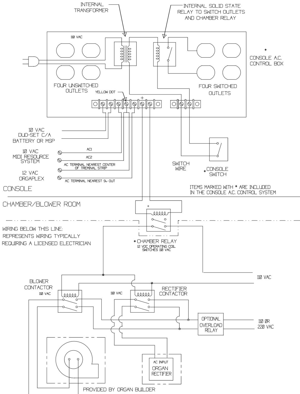
CACC II WIRING DIAGRAM WITH 110V A.C. COILS
