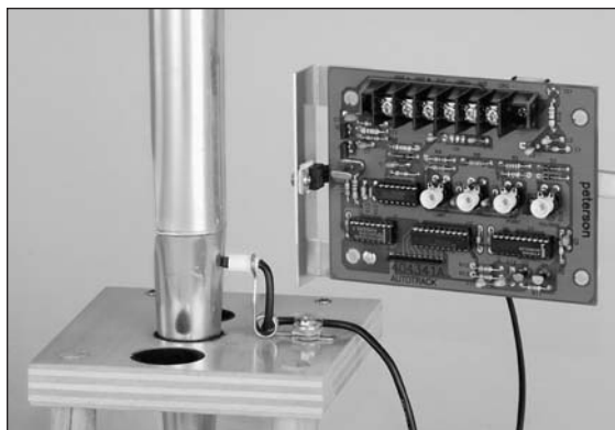
Optional AutoTrack™ includes a temperature sensor in a spring loaded holder.
