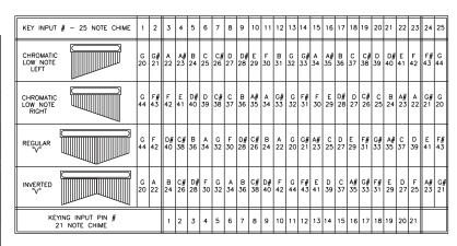
For your convenience in wiring the keying inputs for your PETERSON CATHEDRAL CHIMES, this chart shows the assignment of notes to each pin on the keying junction for four popular configurations.
